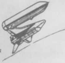
SEPARATION OF EXTERNAL TANK
